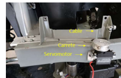
Freno: servomotor, carrete y cable
